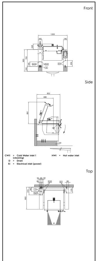
Electric Supply voltage: 400 V/3N ph/50/60 Hz Total Watts: 15.5 kW Installation: FS on concrete base;FS on feet;On base;Standing Type of installation: against wall
